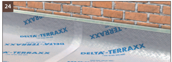
(Fig. 23 and 24) Make sure that sheet overlaps are adequate. Overlap zones should be covered by a double layer of filtration cloth. To make an overlap, push the connecting sheet underneath the raised lateral cloth edge. Simply pull off the backing paper of the adhesive strip and glue the two dimpled sheets together.
