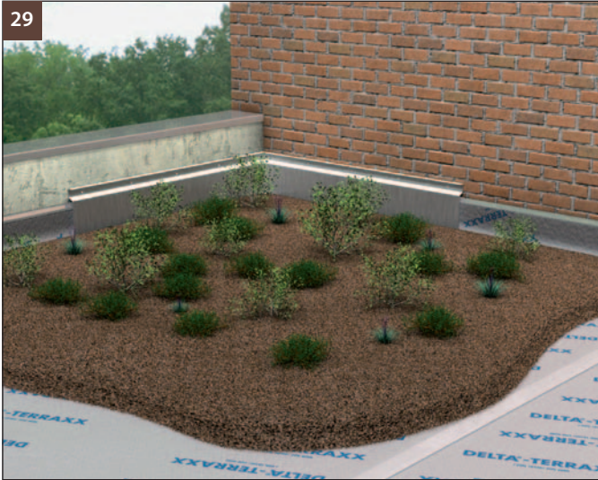
(Fig. 29) For green roofs, the planting substrate may be applied directly in the requisite thickness and planted as required. If a roof is to be planted extensively for low maintenance, substrate thicknesses should range between 8 and 15 cm. If it is to be planted intensively, the substrate should be applied in thicknesses ranging from 20 cm to 100 cm, depending on the plants. Normally, such a roof would require additional irrigation.
